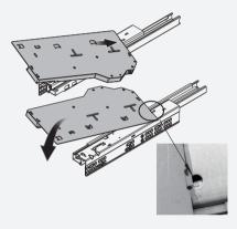
1. Put the push-open mechanism head hook insert to the hole in the bottom slide
